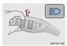
When turning on low beam light, pull combination switch away from steering wheel side and release, headlight high beam comes on; Pull combination switch towards steering wheel side and release to turn off headlight high beam.
