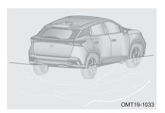
The vehicle could be seriously damaged when driving on a road that has flooded after heavy rain. If driving through water is unavoidable, check the depth of the water and drive slowly and carefully.
