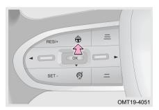
Activate/deactivate function: When ESP is turned on, and TJA/ICA is in pre-activating or activating state, short press TJA/ICA switch to activate/deactivate TJA/ICA.
