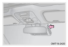
Rear view mirror base USB port can be used for driving recorder.
