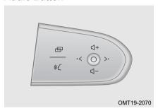
Voice recognition button " « ( ": Short press to wake up the voice recognition function; Long press to wake up the voice assistant (It is necessary to connect with phone).
