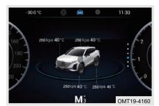
Steering wheel left combination button " | " / right combination button " | " can be used to switch to tire pressure display screen.
