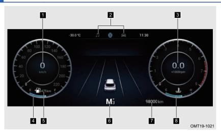
Speedometer: Current driving speed (unit: km/h).
