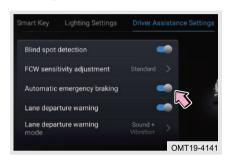
Turn vehicle power to ON mode, and turn on the AEB/FCW in Audio System - Vehicle Settings - Driver Assistance Settings.
