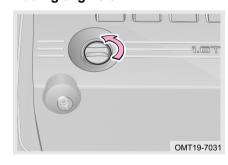
Step 1: Turn the engine oil filler cap counterclockwise to open it;
