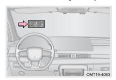
The head up display is located in the front windshield area.
