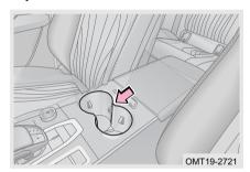
Front cup holder is located on the auxiliary fascia console.
