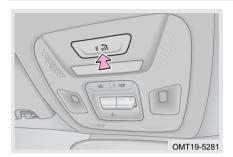
Manual activation: When required to report a serious accident, or require emergency help, manually press the SOS button.
