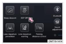
Press ESP OFF switch on the audio system to turn off ESP; Press ESP OFF switch again to turn on ESP.
