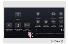
Turn vehicle power to ON mode, press parking radar switch or shift lever is moved to R position, parking radar system is activated, each time the parking radar system is activated, if the parking radar system is normal, it alarms for 0.5 s, parking radar system status indicator comes on and system starts detecting distance at the same time; When a radar sensor detects an obstacle, audio system will display distance from obstacle (red, yellow, green areas) accompanied by alarm sound.
