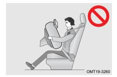
Alwavs keep SRS airbag deployment path clear. It is forbidden to place anything (such as mobile phone) between the occupant and the SRS airbag and fix or place any objects on or near the SRS airbag cover: If there is an object between occupant and SRS airbag, the SRS airbag may not deploy according to design path, or the SRS airbag may push object to occupant's body, causing serious injury or even death.
