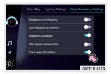
Turn the vehicle power to ON mode, and turn on drive away information system in Audio System - Vehicle Settings - Driver Assistance Settings...
