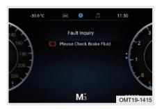
Step 1: On setting screen, press confirmation button up or down to fault inquiry. Short press confirmation button to enter fault inquiry;
