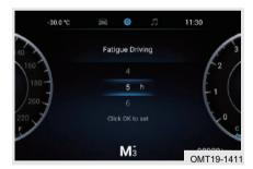
Step 1: On setting screen, press confirmation button up or down to select fatigue driving. Short press confirmation button to enter fatigue driving screen.
