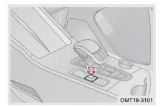
With engine starts or vehicle power is switched to ON mode, depress the brake pedal and press electric parking brake button manually, "(P)" red indicator in instrument cluster and electric parking brake button indicator will turn off, indicating parking brake function has been released.
