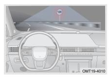
After SLA detects speed limit sign information on road in front and combines the information with speed limit information of navigation system, "20" indicator in instrument cluster remains on, if the speed exceeds current speed limit for 5 km/h, prompt sound will sound 1 time.
