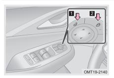
In the vehicle, press lock/unlock switch to lock/unlock the doors.
