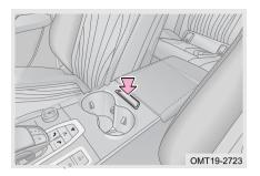
Press the switch and lift the lid to open the auxiliary fascia console storage box.
