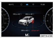
When vehicle power is turned to ON from OFF, and tire temperature is higher than 85°C, system will warn for high temperature. During high temperature warning, corresponding wheel icon and current tire temperature value will be displayed in red and "(!)" yellow indicator in instrument cluster remains on.
