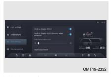
Head-up display (HUD): ON / OFF; Set the steering wheel adjustment HUD on/off, brightness adjustment, height adjustment, snow mode on/ off, Head-up display information display and default value restoring.
