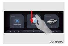
Turn vehicle power to ON mode, slide down the audio screen to display shortcut menu screen and fault inquiry information.
