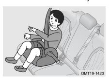
For larger children that cannot fit in a child restraint system with a high back, they may occupy a second row outboard seat using a booster seat. either attached to the lower anchorage points or belted, as described in the instructions provided bν restraint the child system manufacturer.
