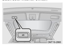
When the power back door opens, press " " switch to close it.
