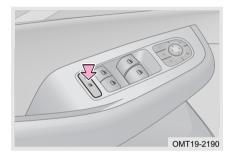
Press passenger side window OFF switch, passenger side window OFF switch indicator comes on, passenger side window switch will be disabled. After disabling, only window switches on driver side can be used to operate passenger side windows (this function is recommended when there is a child in vehicle). Press the switch again to cancel this function and the indicator goes off.
