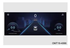
When switching to super sport mode, the starting speed will be accelerated, the simulated sound wave in the driver's room will start, and the mode interface on the audio display will show the steering wheel Angle, turbo value, speed, throttle opening, simulated track, simulated race car, etc.
