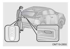
Method 1: With central control lock unlocked, approach the back of vehicle and press exterior switch, on the back door, turn signal lights will come on and power back door will be opened/closed.
