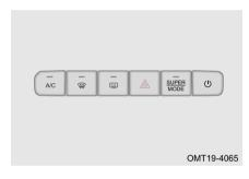
Press drive mode switch, switch among ECO mode, NORMAL mode, SPORT mode or Super sport mode (if equipped). You can choose according to different road conditions. And the corresponding mode icon on instrument cluster will turn on and accompanied by voice reminder to prompt you that driving mode is switched successfully.
