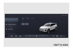
Turn vehicle power to ON mode, and the vehicle is stationary or safe to drive. Manually select driving mode through Audio System - Vehicle Settings - Quick Control; And the corresponding mode icon on instrument cluster will turn on and accompanied by voice reminder to prompt you that driving mode is switched successfully.
