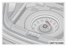
Step 2: Rotate fixing device of spare tire counterclockwise to remove it, and then take out spare tire.
