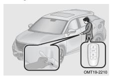
Method 1 (if equipped): Touch the lock sensing area with fingers when carrying smart key on your person, the system automatically recognizes smart key and doors automatically lock.
