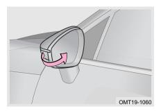
Hold the outside rear view mirror, and push it backward firmly and slowly (-Force increases gradually), until it folds to its position; Hold edge of the outside rear view mirror, and pull forward slightly, until it extends in place.
