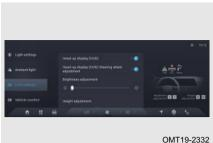
and turn on HUD through Audio System - Vehicle Settings - HUD settings, and set steering wheel adjustment HUD on/ off, brightness adiustment. heiaht adjustment. snow mode on/off. HUD information display, and restore default values.
