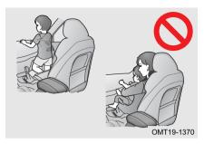
Make sure the shoulder belt is positioned across the center of child's shoulder. The belt should be kept away from child's neck, but not falling off child's shoulder. Otherwise, the child is at risk of serious injury or even death during a collision.
