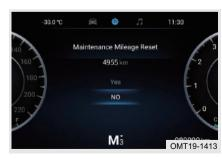
Step 1: On setting screen, press confirmation button up or down to maintenance mileage reset. Short press confirmation button to enter maintenance mileage reset screen.
