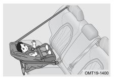
A rearward facing child restraint is installed to face to the rear of the vehicle. Only install a rearward facing child restraint on the front passenger seat if the airbag is OFF. It is recommended children use a rearward facing child restraint system up to 4yrs old.
