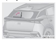
Step 1: Lift the rear wiper arm and hold:
