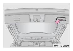
Pull the back door assist handle down and release it before it is fully closed. Make sure the back door is fully closed before leaving the vehicle.
