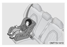
A forward facing child restraint is installed to face to the front of the vehicle. It is recommended children use a forward facing child restraint system when older than 4yrs old.
