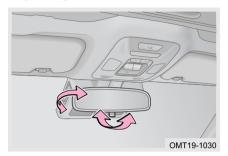
Adjust inside rear view mirror to a proper position before driving, to make sure driver can achieve an optimum view.
