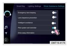
Turn vehicle power to ON mode, and turn on the intelligent cruise control exit reminder in Audio System - Vehicle Settings - Driver Assistance Settings.
