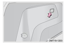
When back door is opened, luggage compartment light will turn on for 15 seconds automatically. When back door is closed, luggage compartment light will turn off immediately.
