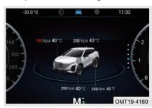
When vehicle power is in ON mode, and tire pressure is less than low alarm threshold, system will warn for low pressure. During low pressure warning, corresponding wheel icon and current tire pressure value will be will be displayed in red and "!!" yellow indicator in instrument cluster remains on.
