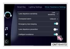
Turn the vehicle power to ON mode, and turn on intelligent avoidance system in Audio System - Vehicle Settings - Driver Assistance Settings.
