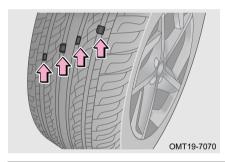
Check the tire tread by tread wear mark. When tread wear reaches its limit, tread will be in the same plane as the wear band. If such condition occurs, the tire performance and safety will be seriously impacted, and replacement is necessary.
