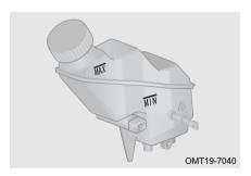
Brake fluid level should be between the "MIN" and "MAX" marks. If the level is at or below the "MIN" mark, add brake fluid and contact the authorized service station for inspection and repair immediately.
