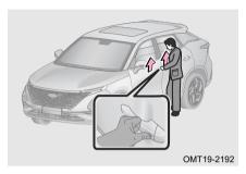
While the window is rising, touch lock sensing area with fingers (-carry smart key on your person), window glass stops rising.
