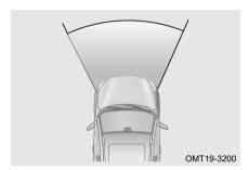
In general, in an event of frontal collision, the driver airbag and front passenger airbag will deploy if the deceleration of vehicle exceeds the designed threshold level.
