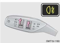
Turn vehicle power to ON mode, when front fog light or low beam lights turn on, operate fog light switch to " 0\(\frac{1}{2}\)# " position to turn on rear fog light; After turning vehicle power to OFF mode or operate fog light switch to " 0\(\frac{1}{2}\)# " or "OFF" position again, rear fog light turns off.
