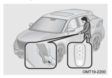
Method 1 (if equipped): Touch the unlock sensing area with four fingers when carrying smart key on your person, the system automatically recognizes smart key and doors automatically unlock.
