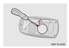
Step 2: Pry off battery cover and battery using a flathead screwdriver with the tip taped;
