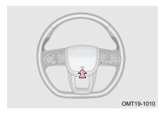
To sound the horn, press area near horn mark on the steering wheel.
